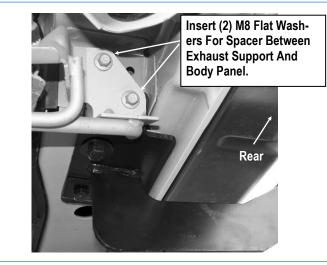
(Fig 11) Passenger Rear Mounting Bracket (09-010 models: Install Mounting Bracket Between Exhaust Support And Body Panel)
