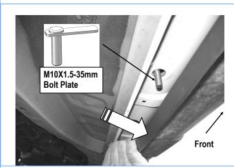
(Fig 3) M10 Bolt Plate Installed (On Driver Side Front Mounting Location)
