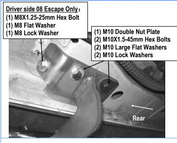
(Fig 10) Driver Rear Mounting Bracket (DRM) Installed
