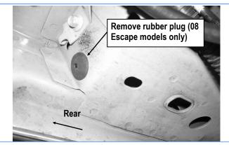
(Fig 8) Driver Side Rear Mounting Location
