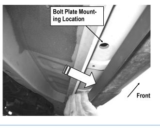
(Fig 2) Driver Side Front Mounting Location
