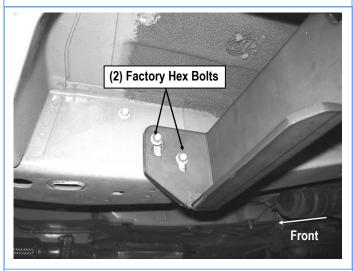
(Fig 5) Driver Front Mounting Bracket (DFM) Installed
