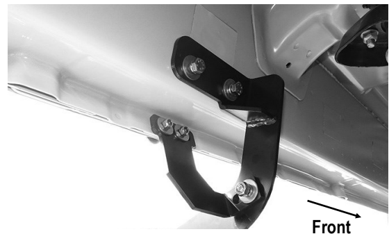
(Fig 11) Driver Side Front Brackets Installation Completed
