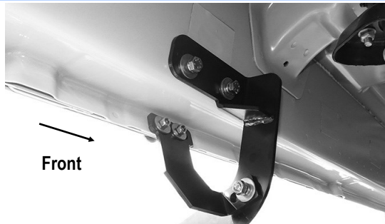
(Fig 12) Driver Side 2nd Brackets Installation Completed
