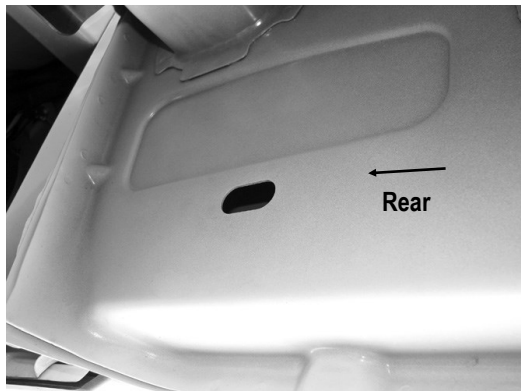
(Fig 14) Driver Side Rear Mounting Location
