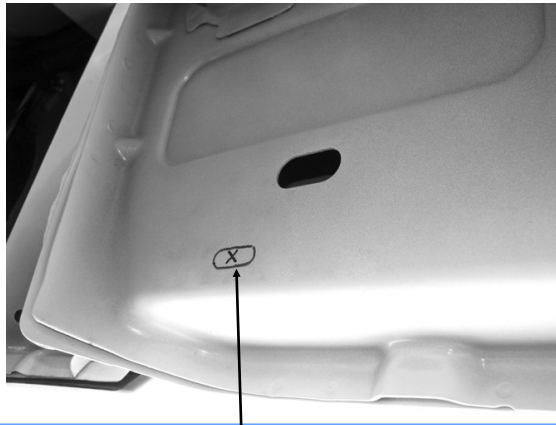
(Fig 17) Use A 7/16" Drill Bit To Drill Hole In Center Of Slot As Marked
