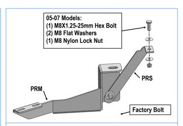
(Fig 5) Passenger Side Rear Brackets Installation (05-07 Models)
