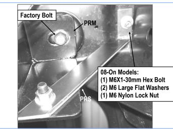
(Fig 6) Passenger Side Rear Brackets Installed (08-UP Models)
