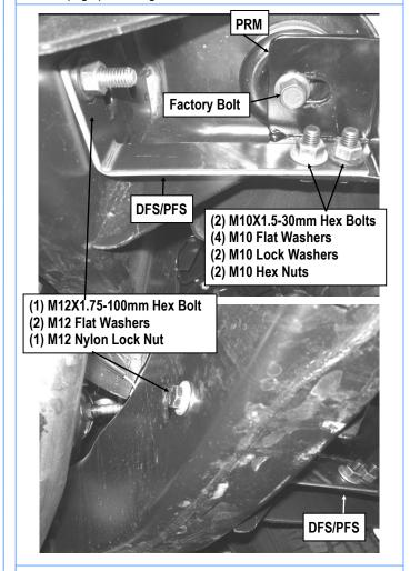
(Fig 3) Passenger Side Front Brackets Installed
