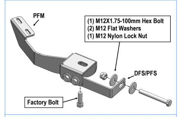
(Fig 2) Passenger Side Front Brackets Installation
