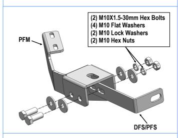
(Fig 1) Passenger Side Front Brackets Assembly
