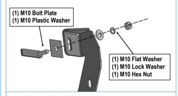
(Fig 15) Driver Front Mounting Bracket Installation
