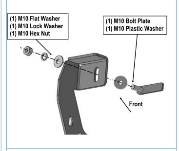
(Fig 4) Passenger Front Mounting Bracket Installation
