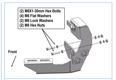
(Fig 10) Attach Support Bracket To Pinch Weld (Passenger Front Mounting Bracket)
