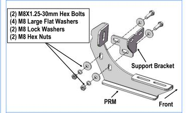
(Fig 8) Passenger 2nd & 3rd & Rear Mounting Bracket and the Support Bracket Assembly
