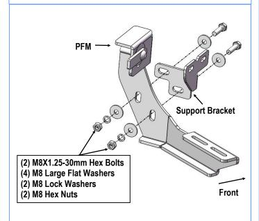
(Fig 5) Passenger Front Mounting Bracket and the Support Bracket Assembly
