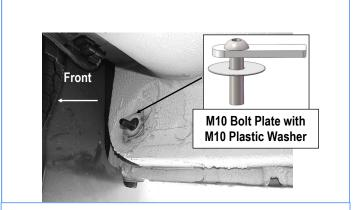
(Fig 3) Insert M10 Bolt Plate
