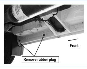
(Fig 2) Passenger Side Front & 2nd Mounting Location
