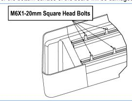
(Fig 11) Slip M6X1-20mm Square Head Bolts Into The Bottom Channels
