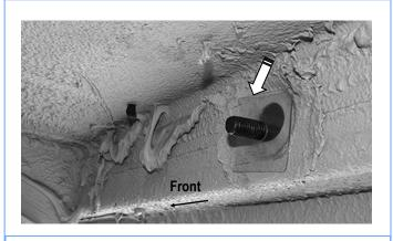
(Fig 7) Inserted The Bolt Plate Into The 3rd Mounting Location
