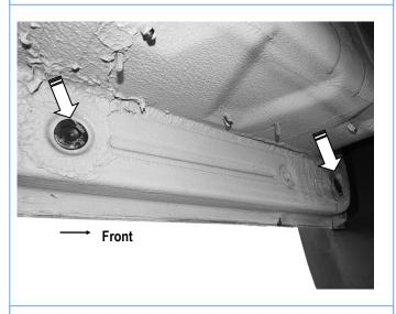
(Fig 13) Driver Side Mounting Locations
