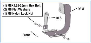
(Fig 2) Driver Front Mounting Bracket and the Driver Front Support Bracket Assembly
