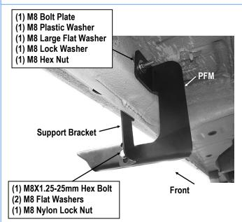
(Fig 11) Passenger Side Front Brackets Installation
