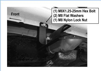
(Fig 9) Driver Side Support Bracket Installed on Pinch Weld
