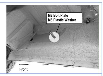
(Fig 10B) Passenger Side Front Mounting Location
