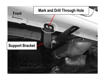
(Fig 8) Mark and Drill Through Holes on Pinch Weld
