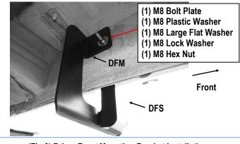
(Fig 3) Driver Front Mounting Bracket Installation
