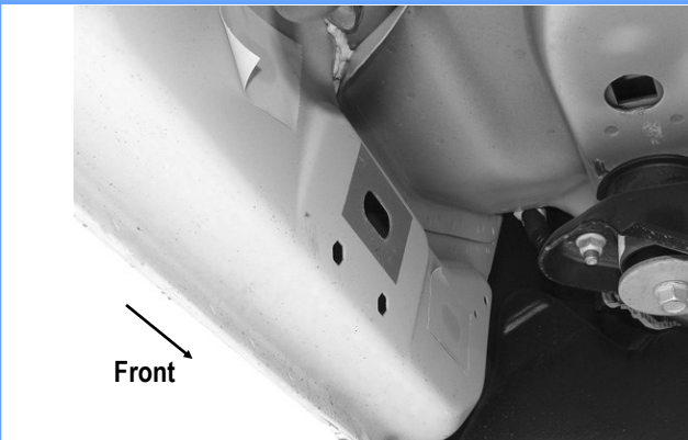
(Fig 1) Driver Side Front Mounting Location (No Factory Holes In Pinch Weld on Some Models)
