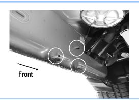
(Fig 1) Driver Side Front Mounting Location
