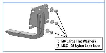
(Fig 4) Driver Front Mounting Bracket Installation
