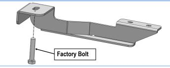
(Fig 1) Driver Front Mounting Bracket Installation
