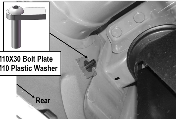
(Fig 14) Insert The M10X30 Bolt Plate
