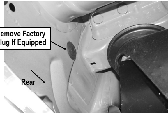
(Fig 13) Passenger Side Rear Support Bracket Location
