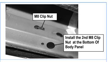
(Fig 3) M8 Clip Nut Installation
