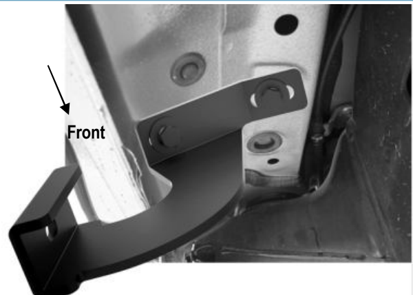
(Fig 4) Driver Front Mounting Bracket Installed
