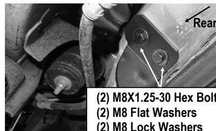
(Fig 7) Driver Rear Mounting Bracket Installed
