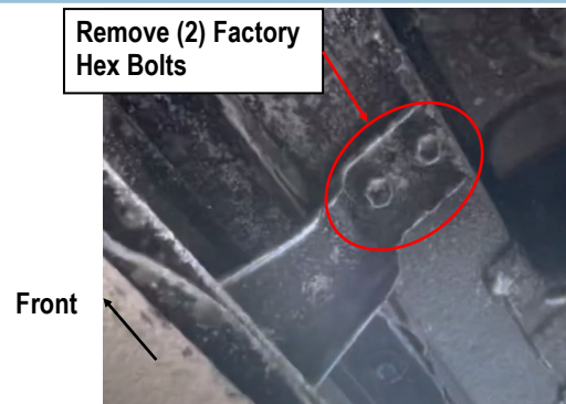
(Fig 3) Passenger Side Center Mounting Location
