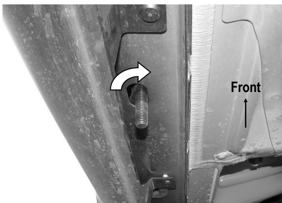
(Fig. 4) Insert The A1 (M10 Bolt Plate)
