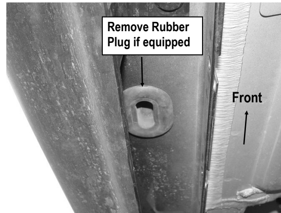
(Fig. 3) Passenger Side Front Mounting Location on Rocker Panel
