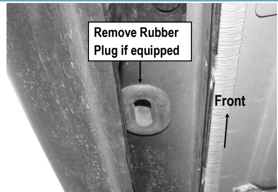
(Fig 2) Passenger Side Front Mounting Location on Rocker Panel
