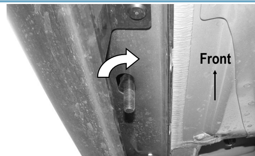
(Fig 3) Insert The M10 Bolt Plate
