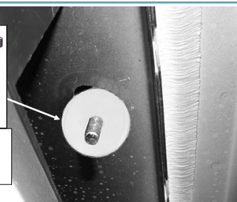
(Fig 4) Thread The Plastic Washer On The Bolt Plate
