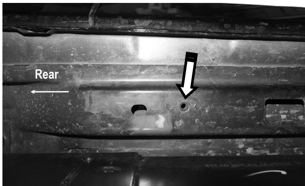
(Fig 5) Passenger Side Rear Mounting Location (Vehicles with factory threaded hole in floor panel)
