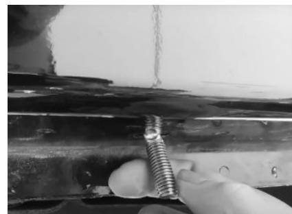
(Fig 3) M10 J-Bolt Installation (On Driver Side Mounting Location)
