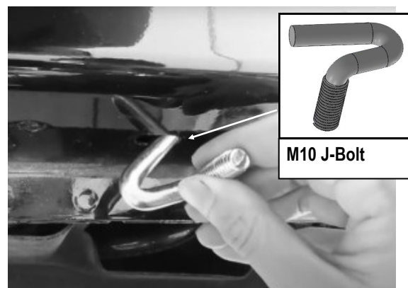
(Fig 3) M10 J-Bolt Installation (On Driver Side Mounting Location)
