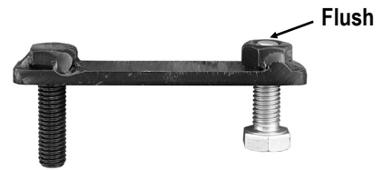
(Fig. 4) Thread M8X1.25-30 Hex Bolt into the welded nut on the plate
