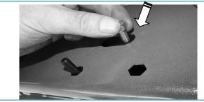
(Fig 4) Use The Loose Hex Bolt As A Handle. Insert The M8 Nut/ Bolt Plate Into The Oval Hole And Feed The Threaded End Out Either Factory Hex Shaped Hole.
