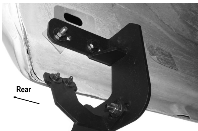
(Fig 12B) Driver Rear Brackets installed
