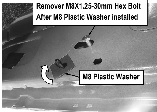
(Fig 5) Thread Plastic Washer Onto the Welded Bolt on M8 Bolt/Nut Plate To Hold Bolt/Nut Plate In Position.
