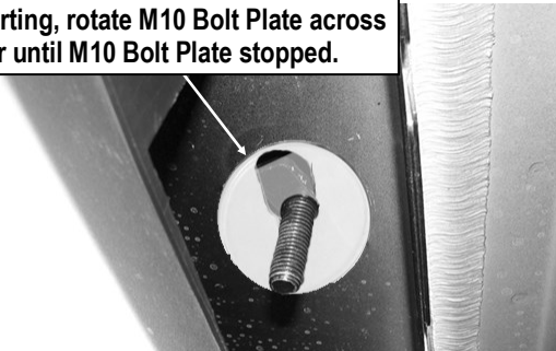
(Fig 4) M10 Bolt Plate Installed on Driver Side Front Mounting Location
