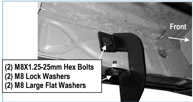
(Fig 6) Driver Side Front Bracket Installed
