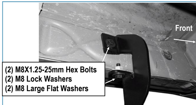
(Fig 6) Driver Side Front Bracket Installed
