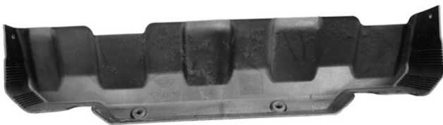
(Fig 13B) 17-UP Passenger side DEF cover removed
