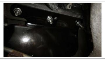
Torque the M12 hardware to 58 ft-lb. Reinstall exhaust and fascia screws from step 1
