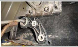
Finish lowering the exhaust by removing the exhaust rubber isolator in front of the muffler.
