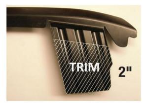
Mark and trim the underbody panel. See the trim diagram for reference. Dimensions are approximate. Confirm fit prior to trimming. Use the ribs of the underbody panel as cutting guides. Reattach the underbody panel using the fasteners removed in Step 1.
