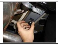
Raise hitch into position and loosely secure hitch with the hardware, careful not to push hardware inside vehicle frame. Trimming of exhaust bezel may be required on some models (Check trim fitment around hitch, additional trimming may 8 be required. Seam foam may need to be trimmed for proper fitment).
