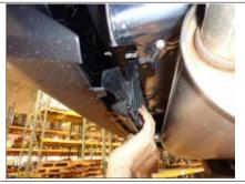
Trim the center of the fascia roughly 3 1/2" by 4 3/4" with a cut off wheel. (see pictures below, removing the fascia is not notrequired fortrimming)
