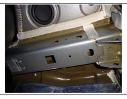
Fishwire the rear and side hardware though access hole in frame, then reverse fishwire the hardware into the access hole (both sides). On Trailhawk models only the reverse fishwire hardware and M14 bolts removed in Step 4 are used.
