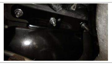
6 Torque the M12 hardware to 58 ft-lb. Reinstall exhaust and fascia screws from step 1
