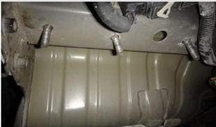
Raise hitch into position and secure the hitch to the vehicle using (6) M12 hex flange nuts.
