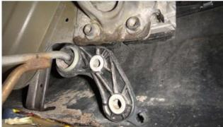
Finish lowering the exhaust by removing the exhaust rubber isolator in front of the muffler.
