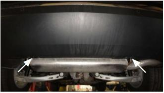
Lower the exhaust by removing the (4) bolts from each of the rear exhaust hanger brackets (2 per side) using a 15mm socket.
