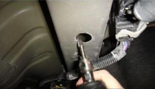
Utilizing the access hole, fishwire (1) M12 carriage bolt and (1) spacer into each of the three mounting holes in both frame rails.
