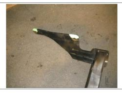
Fishwire M12 carriage bolt with spacer in through access hole and out rearmost mounting location in the passenger frame rail. Repeat on rearmost mounting location in driver side frame rail (if there is no weldnut in frame). Leave hardware fully inside of frame rail(s) with fishwire(s) attached. See FISHWIRE TECHNIQUE diagram on page 2.
