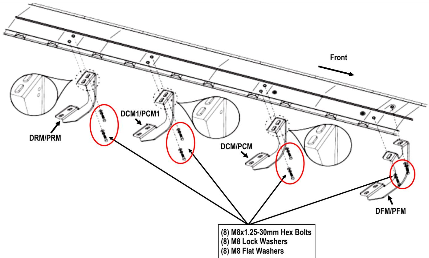
(Fig 1) Driver Side Mounting Brackets Installed
