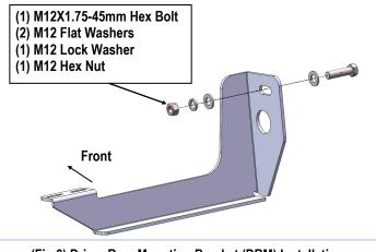
(Fig 6) Driver Rear Mounting Bracket (DRM) Installation
