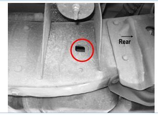
(Fig 5) Driver Side Rear Mounting Location
