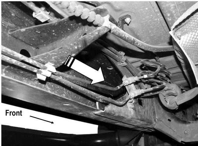
(Fig 2) M12 Long Bolt Plate Install Location
