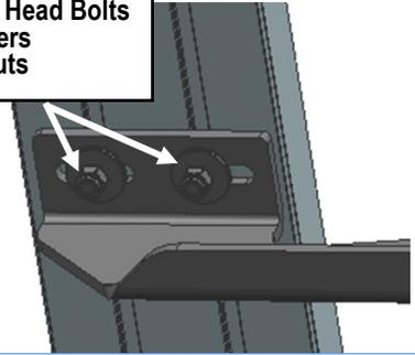
(Fig 6) Running Board Installed Onto Mounting Bracket
