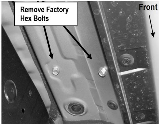
(Fig 1) Passenger Front Mounting Bracket Location Pictured
