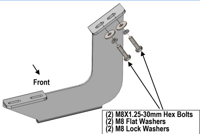
(Fig 4) Driver Center/Rear Mounting Brackets Installation
