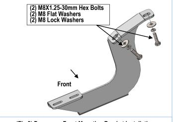
(Fig 2) Passenger Front Mounting Bracket Installation
