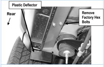
(Fig 3) Passenger Rear Mounting Bracket Location Pictured
