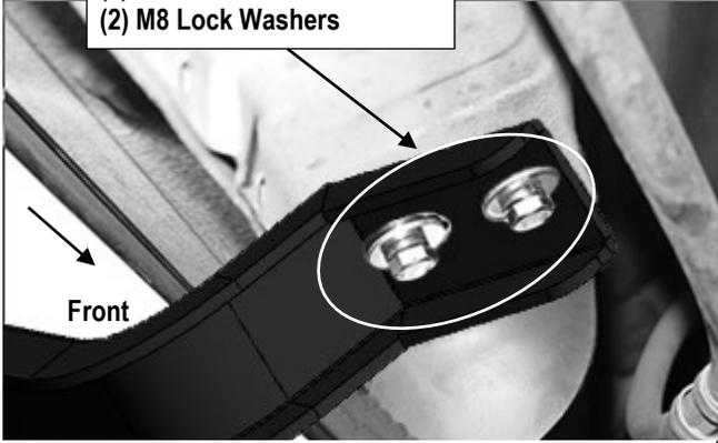
(Fig 4) Driver Rear Mounting Bracket Installation Pictured
