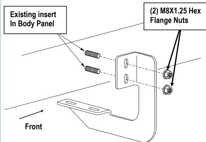
(Fig 1) Driver Side Front Mounting Bracket Installation
