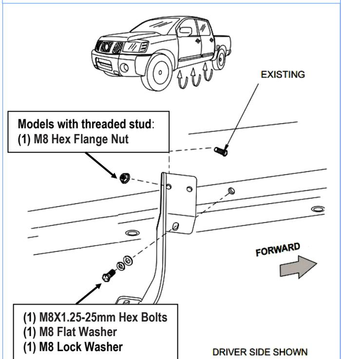
(Fig 3) Models With Threaded Stud Bracket Installed
