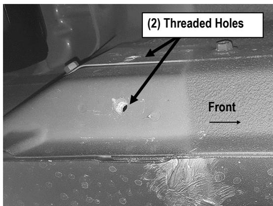
(Fig 2) 2016-On Driver Side Rear Mounting Location Pictured.
