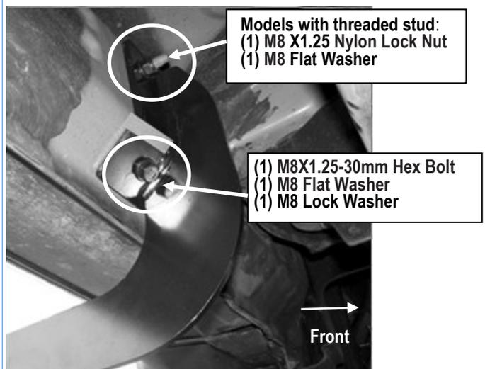
(Fig 3) Models With Threaded Stud Bracket Installed
