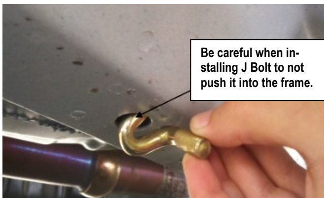
(Fig 2) Install M10 J-Bolt (on Driver Side Front Mounting Location)
