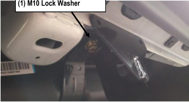
(Fig 8) Driver Rear Mounting Bracket Installed
