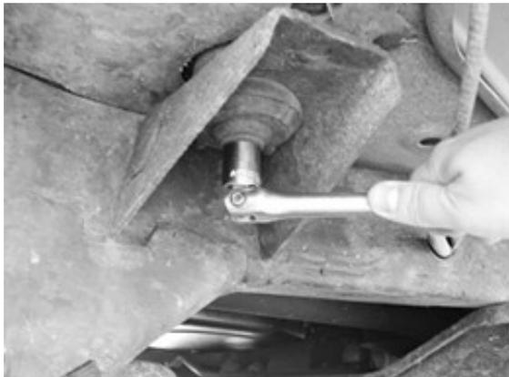
(Fig 1) Remove Factory Body Mount Bolt
