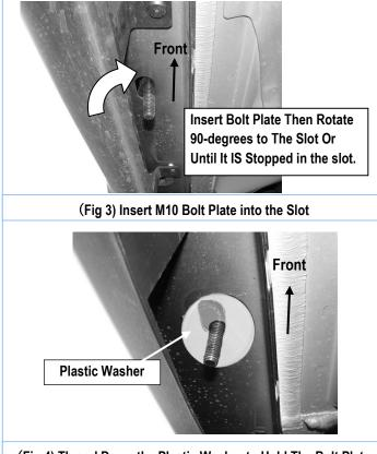
(Fig 4) Thread Down the Plastic Washer to Hold The Bolt Plate
