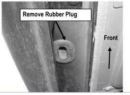
(Fig 2) Remove the Rubber Plug (At the bottom of the Rocker Panel)
