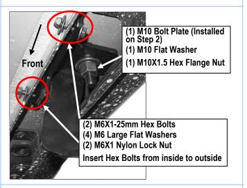
(Fig 5) Passenger Front Mounting Bracket Installation
