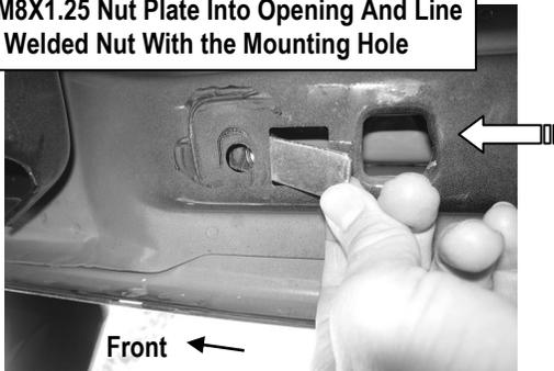
(Fig 1) Vehicle with opening In Floor Panel (Passenger Side-Front Mounting Location)
