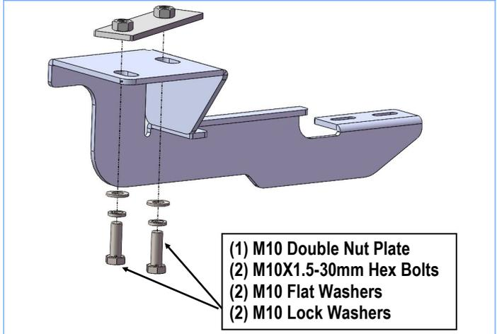
(Fig 2) Driver Front Mounting Bracket (DFM) Installation
