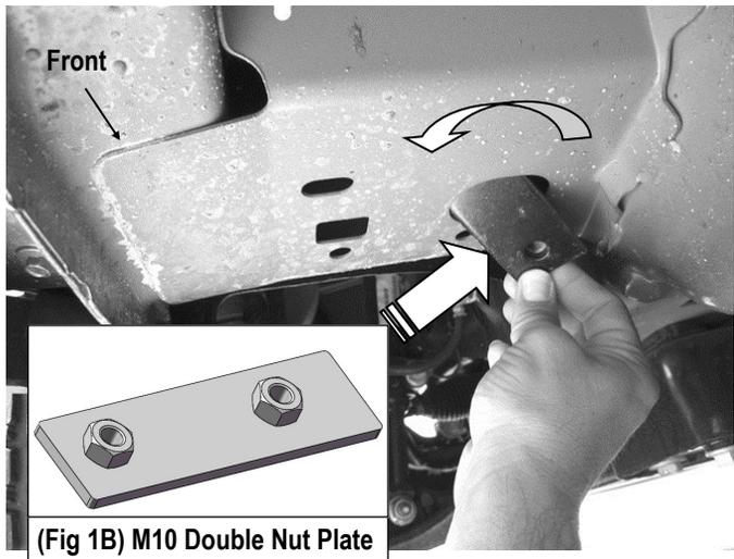
(Fig 1A) M10 Double Nut Plate Installation
