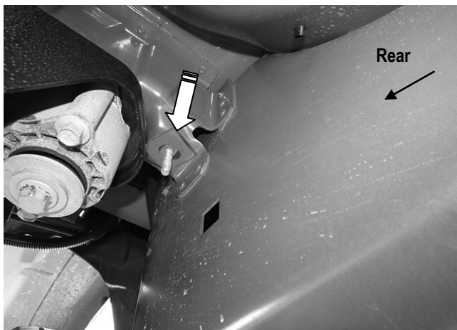
(Fig 8) Insert T-Bolt and folded Washer into oval hole. Thread second Plastic Washer onto T-Bolt
