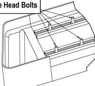
(Fig 4) Slip M6X1-20mm Square Head Bolts Into The Bottom Channels
