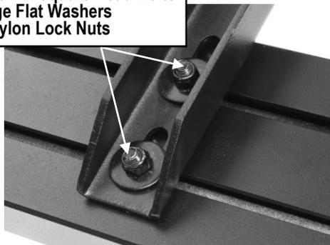
(Fig 6) Running Board Installed Onto Mounting Bracket
