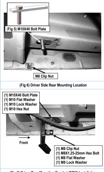
(Fig 7) Driver Rear Mounting Bracket (DRM) Installation
