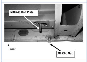
(Fig 12) Passenger Center Mounting Bracket (PCM) Location
