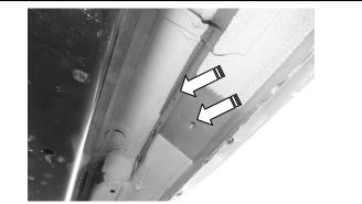
(Fig 3) Passenger Center Mounting Location Pictured
