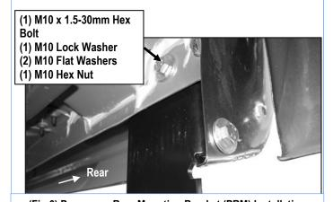
(Fig 6) Passenger Rear Mounting Bracket (PRM) Installation
